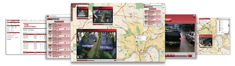
Livetrax is a powerful, web based, live video streaming and fleet tracking service designed for Safety Vision DVRs. Livetrax utilizes cellular networks to stream video on-demand to authorized users via simple browser interface. Livetrax is architected with scalability in mind to support any sized fleet with simultaneous streaming from multiple vehicles, real time fleet tracking, intuitive historical mapping, reporting and more in one simple service.
